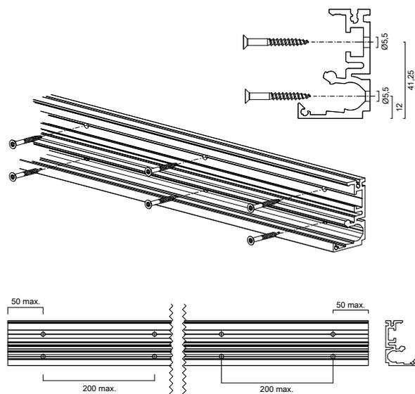
Drill position for assembly of base profile to case:
